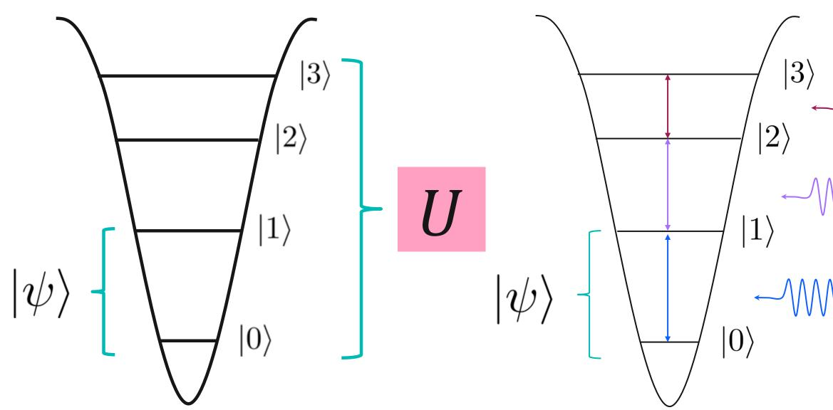
Using superconducting qubits as anharmonic oscillators (can also be applied to other quantum computing architectures whenever qubits are embedded in larger spaces and extra degrees of freedom are accessible)
